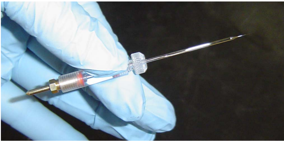
Figure 13: Microelectrode assembly with glass capillary in place.
